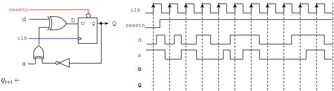
Complete the timing diagram of the circuit shown below. Get the excitation equation for Q (10 pts)
